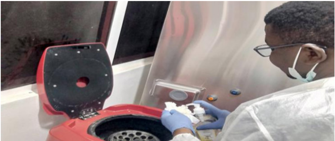
Figure 8: Calibration of Bucket Centrifuge In ACE-5 Supported Facility
